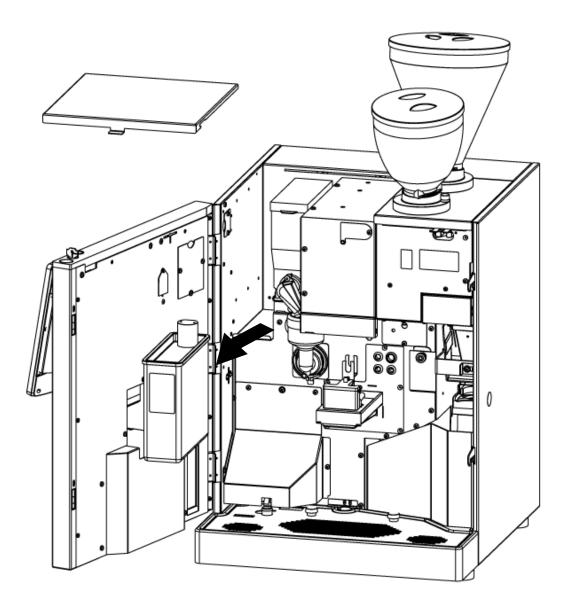
Now it is necessary to remove the tank from the machine. To extract it, you need just to pull it to toward yourself.
