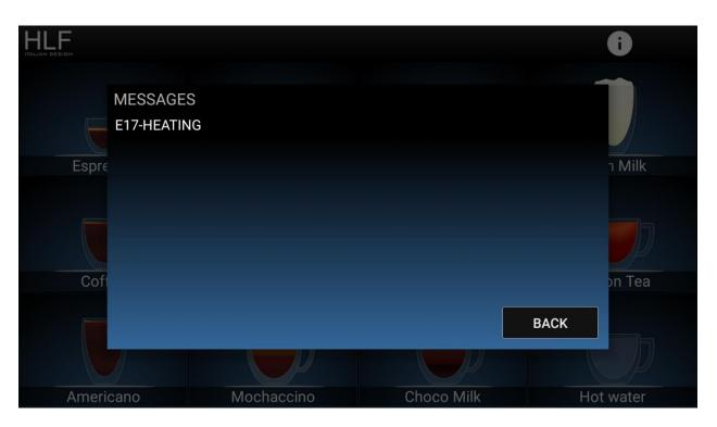
The internal boiler is heating the water, and this process should take around 5 minutes. When the notification icon disappears, the machine is ready to work.
