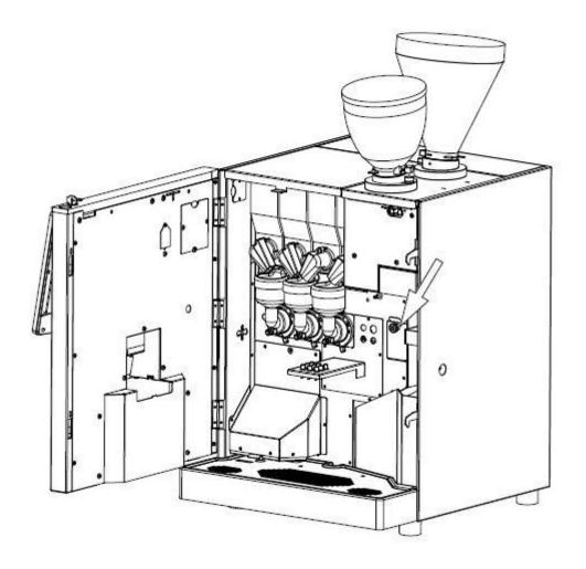
Open the door and unscrew the knob indicated in the picture.
