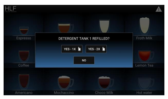
Choose the correct quantity of detergent refilled (assuming the capacity of a bottle of detergent is 1000ml), insert the password (default is **123456**, you can edit or disable it in *Main Menu > Security*), and the alarm will disappear.
