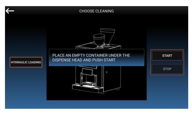
Push on the **Start button** to start the Hydraulic Loading procedure. This operation will take about 5 minutes.
