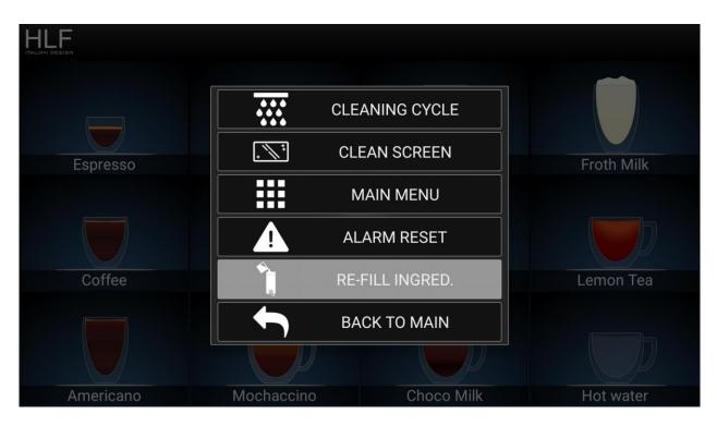
Access the Re-Fill Ingredients section during the <u>first installation of the machine</u> in order to set parameters for each product container.
