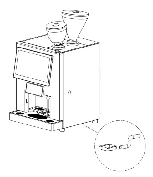
Then make a hole (diameter 7 mm) in the plastic drip tray (see image below). In this way the liquid collected, will be discharged externally through the tube that was previously connected (previous step).
