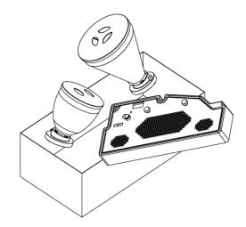
Extract the coffee hopper/s from the box and install it in the neck on the top lid of the HLF 5700 coffee machine, turn it clockwise until the micro fits into the hole (see image below).
