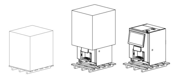
Along with the HLF 5700 package, is provided also a second box containing the external coffee beans hopper/s and the drip tray.
