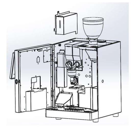
Lift the lid of the tank and disconnect the connection pipe from the tank.
