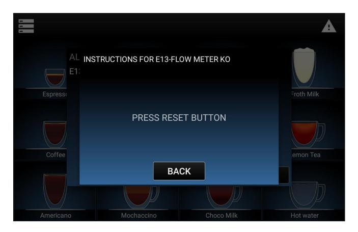
After the press of the RESET button the machine will load the boiler, and the Hydraulic
