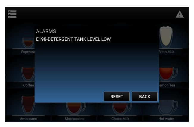
When the detergent tank needs to be refilled, you will see this alarm in the main screen:
