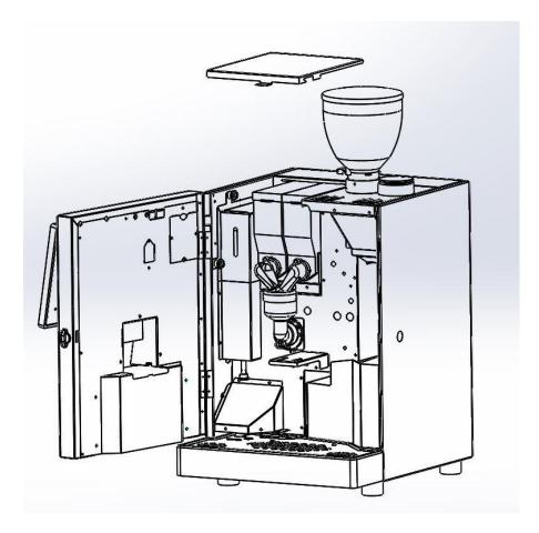
Take off the top lid, open the front door and screw the knobs on the left. Remove the top of the tank (as the image below)
