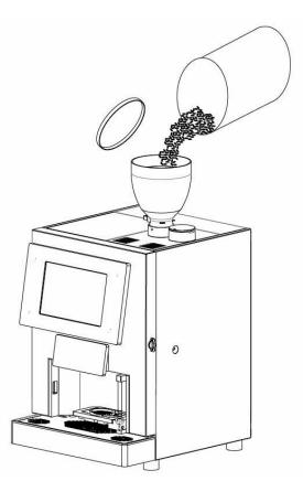
Remember to open the beans stopper located at the bottom of the coffee beans hopper. (see image A below).
