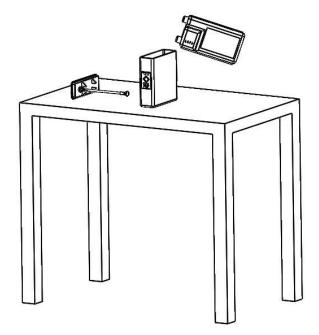
When the tank is empty, reposition it and put the lid on and screw the knobs.
