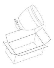
Extract the coffee hopper/s from the box and install it in the neck on the top lid of the HLF 2700 coffee machine, turn it clockwise until the micro fits into the hole (see image below).
