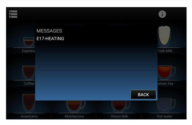
The internal boiler is heating the water and this process is going to take around 5 minutes. When the notification icon disappears, the machine is ready to work.
