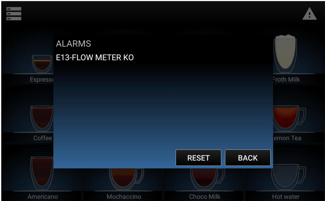
Push on the **FLOW METER KO** alarm and the following screen shot will appear. This happened because at the first initial water fill in of the machine, the water doesn't arrive directly to the boiler.
