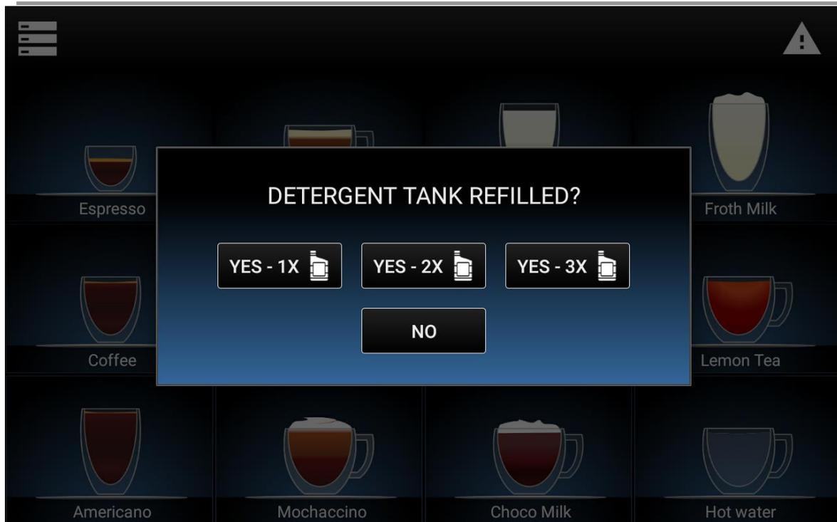
Choose the correct quantity of detergent refilled (assuming the capacity of a bottle of detergent is 1000ml), insert the password (default is **123456**, you can edit or disable it in *Main Menu > Security*), and the alarm will disappear.
