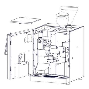
Take off the top lid and open the front door. Before to lift the tank, disconnect the grey tube from it (as the image below).
