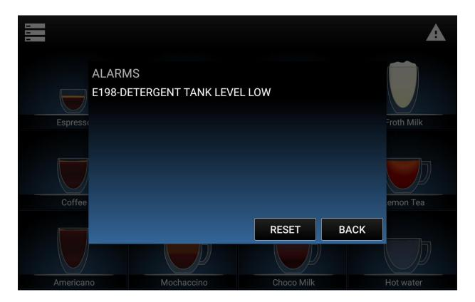
If the alarm is still showing, press on the **Reset** button to show the detergent tank refill request.
