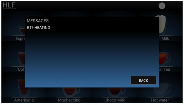
The internal boiler is heating the water, and this process should take around 5 minutes. When the notification icon disappears, the machine is ready to work.
