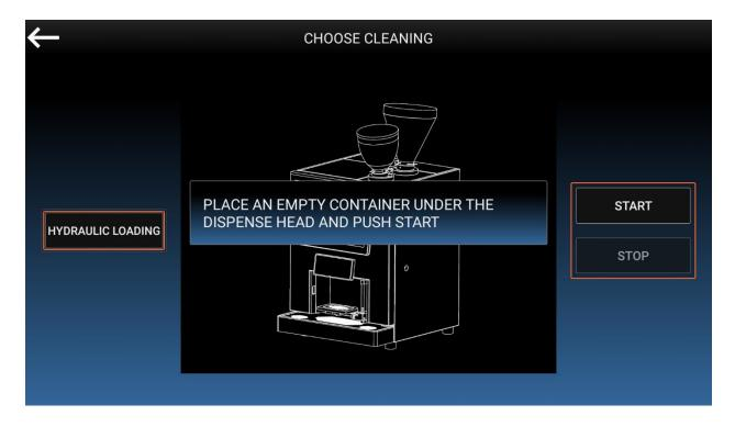
Push on the **Start button** to start the Hydraulic Loading procedure. This operation will take about 5 minutes.
