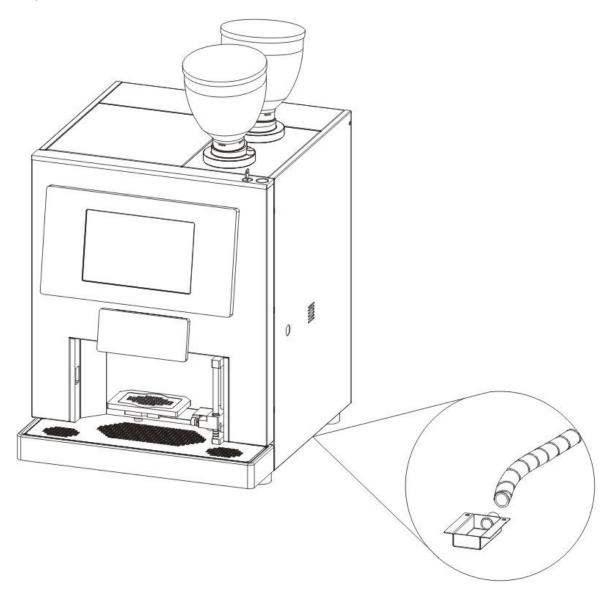
Then make a hole in the plastic drip tray (see image below). In this way the liquid collected, will be discharged externally through the tube that was previously connected (previous step).
