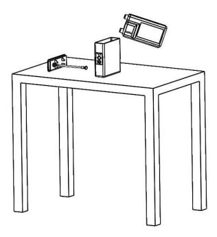
Refill the tank as the image and when it is empty, reposition the tank, connect the grey tube, and close the door.
