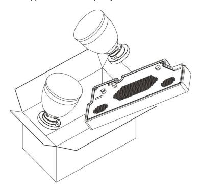
Extract the coffee hopper/s from the box and install it in the neck on the top lid of the HLF 5700 coffee machine, turn it clockwise until the micro fits into the hole (see image below).
