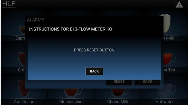
This happened because at the first initial water fill in of the machine, the water doesn't arrive directly to the boiler.
