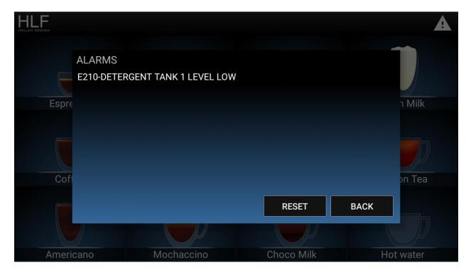
Press on the **Reset** button or open the door, refill the detergent tank and close the door.
