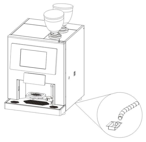
Then make a hole in the plastic drip tray (see image below). In this way the liquid collected, will be discharged externally through the tube that was previously connected (previous step).
