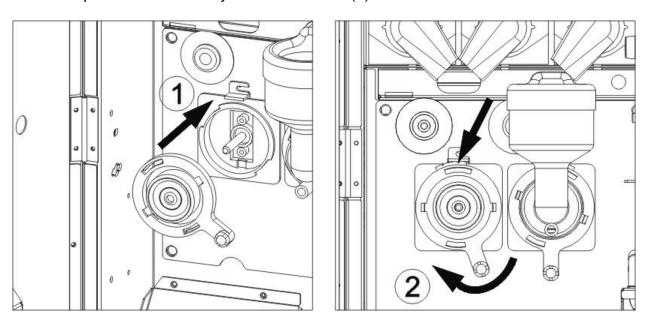
2. mixing blade turn the shaft with the flat side up (1) and insert the mixing blade so that its internal flat side aligns with the one of the shaft.
