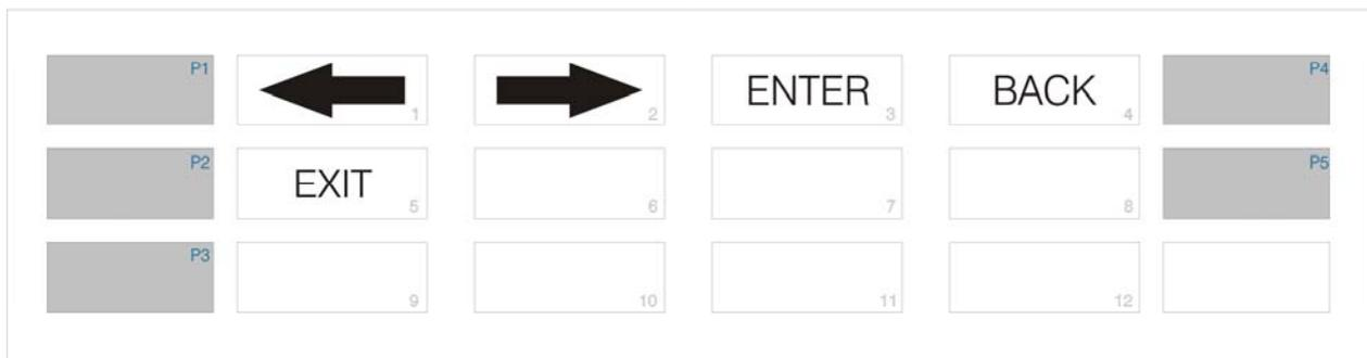
Buttons 1 and 2 are used to move forward or backward through the various programming functions. These buttons are also used to decrease and to increase the various product doses and water amounts.
