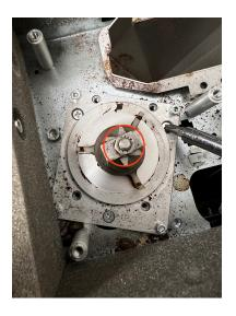
If replacement of the gear is needed, remove the lower blade from the spindle with a 10mm socket. Note: this is a reverse thread. Turn clockwise to remove.
