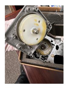
You can now lift the top of the grinders and inspect the white plastic gear.
