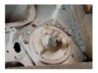
This gear is only found in the modules with conical blades.
