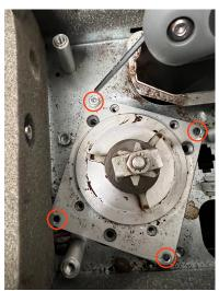
then these four allen head screws that connect the grinder motor to the module.
