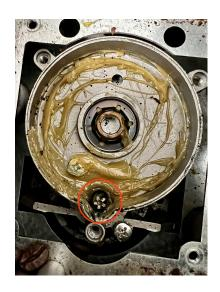
Before reassembly, check for and remove any bits of plastic broken off the white gear that may be trapped in the grease - especially in the marked area.
