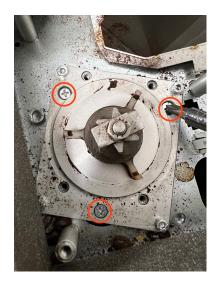
Next, remove these three screws that hold the grinder together,
