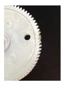
Early versions of the grinder module (those using conical blades) used a white plastic gear to connect the grinder motor to the blades.
